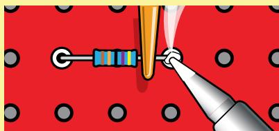
**Measuring and soldering leads.** When installing the resistors and capacitors, span the connections you will be making and trim the leads an extra 1/4" longer on each end than they need to be. Precisely measure the distance and bend the leads to fit. Insert the bent ends into the holes on top of the turrets as shown.
