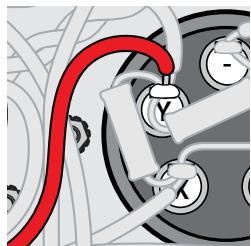
Next, solder the output transformer primary wires to the appropriate locations. First, measure the
