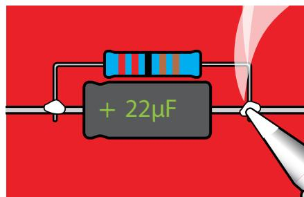
Next, center the 1.8K resistor 1/8" away from one of the 22uF capacitors and wrap the resistor leads around the capacitor leads where they intersect. Solder the leads in place. The result should be the resistor "piggybacking" the capacitor.
