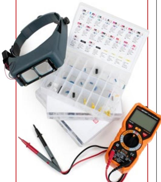
Identifying numbers, letters and color bands on parts isn't always easy. To make the process more efficient, we've sorted the smaller parts into a couple of tackle boxes. However, we recommend always having both a magnifying device and a multimeter on hand.
