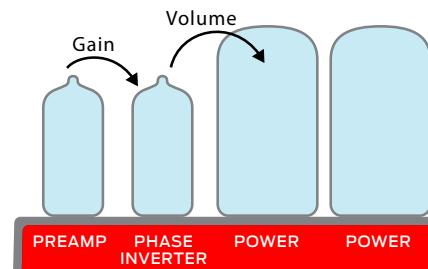
The volume knob sets the level of signal from the final preamp stage to the power tubes. While keeping the tone you found with the gain knob, volume makes it louder or softer. Play with these two knobs to dial in a gritty tube crunch at lower volumes.
