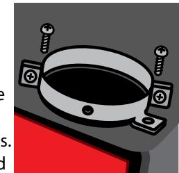
This step is important, as we need to leave enough clearance to allow for the IEC power inlet to be installed without interference, and to permit dressing the associated wiring around and above the large can capacitor.
